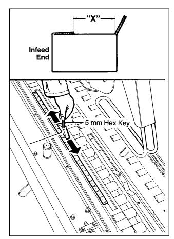
Figure 3-8 – Box Size Set-Up
